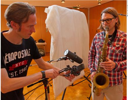
Although the sax 'peer-array' mic (an AKG C414 B-XLS) and the alternative spot mic (a Shure SM7B) were positioned very close together, the former's omni polar pattern delivered a significantly more natural sound — albeit at the expense of more spill and room ambience.
