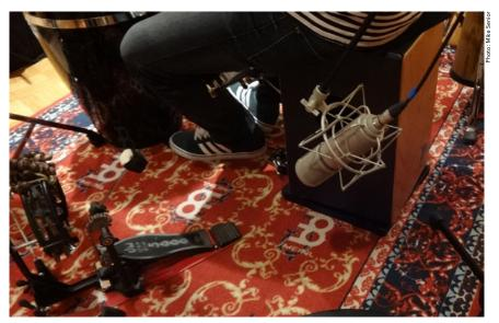
As part of the percussion 'peer-array' setup, an sE Electronics Z3300A was set up in figure-of-eight mode to cover the cajon.
